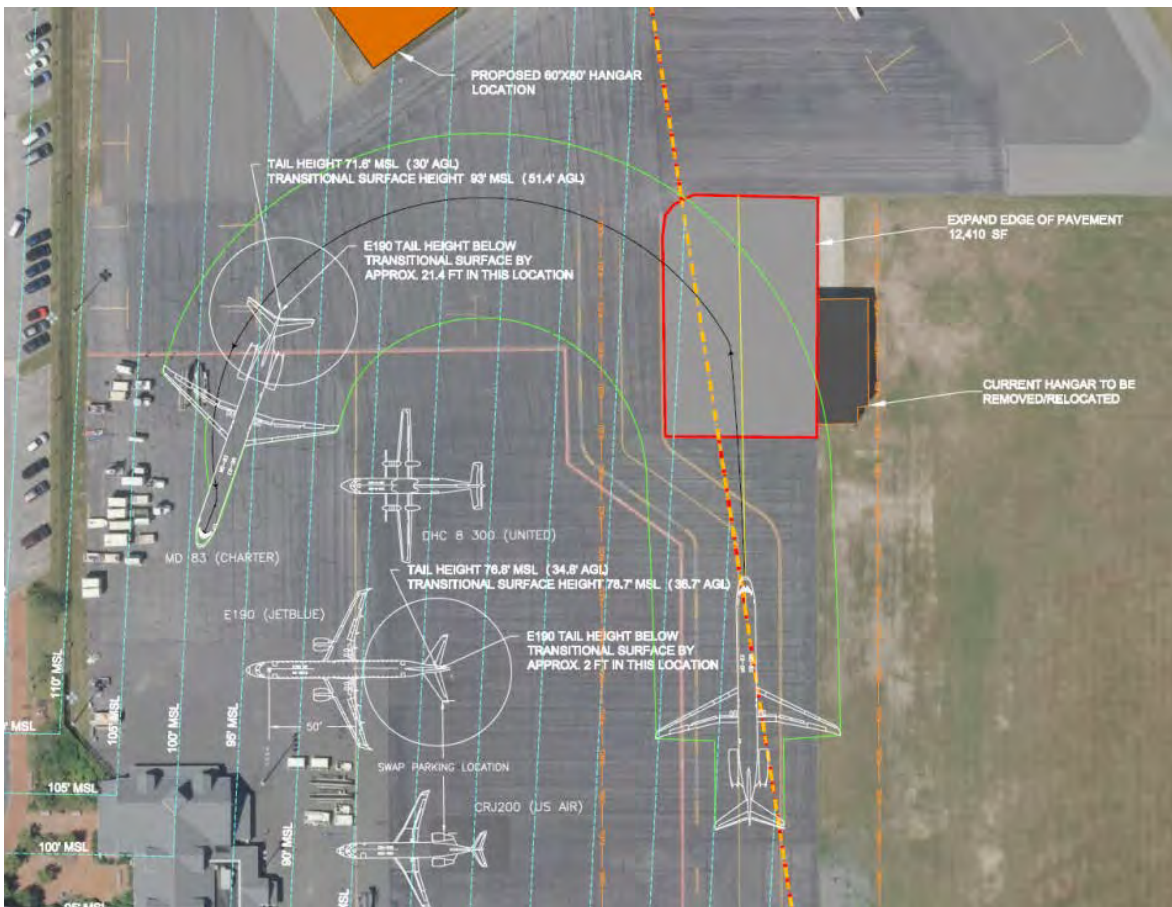
Figure 7-23 Alternative 1- Create New Parking Position - RECOMMENDED
