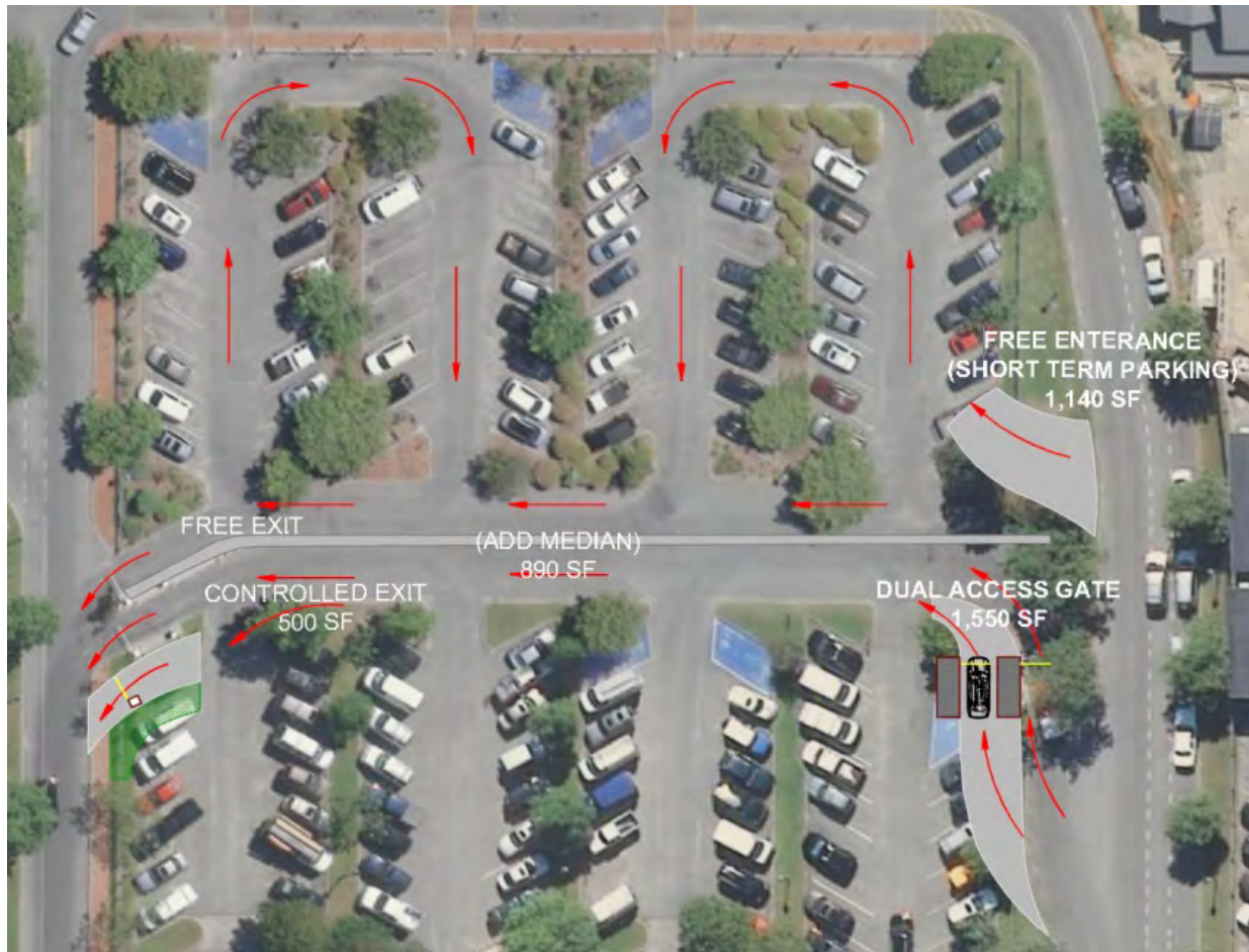
Figure 7-40 Free Short-term Access/2 nd Control Gate/Median Barrier - RECOMMENDED
